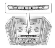
The power door lock switches are on the instrument panel.
